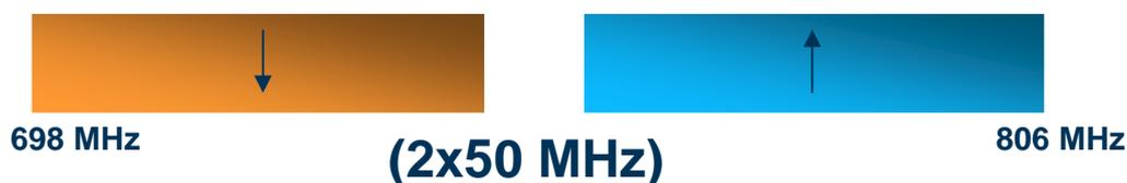
Figure 3. A 2x50 MHz arrangement between 698-806 MHz with an 8 MHz gap between downlink and uplink directions
