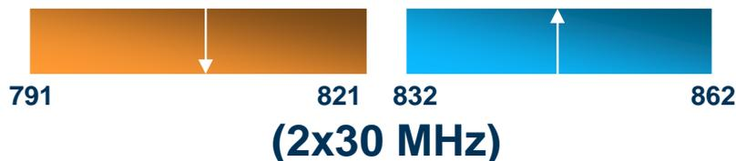
**Figure 1** 791 – 821 MHz D/L frequency is paired with 832 – 862 MHz U/L frequency using reversed duplex. 30 + 30 MHz FDD with 41 MHz duplex separation and 821 – 832 MHz (11 MHz) as the centre gap.
