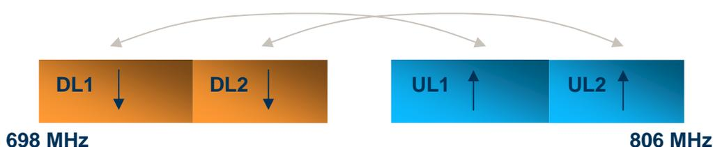
Figure 4. A solution with dual duplexers having the same duplex distance that could be of same or different sizes (DL1 paired with UL1 and DL2 paired with UL2)
