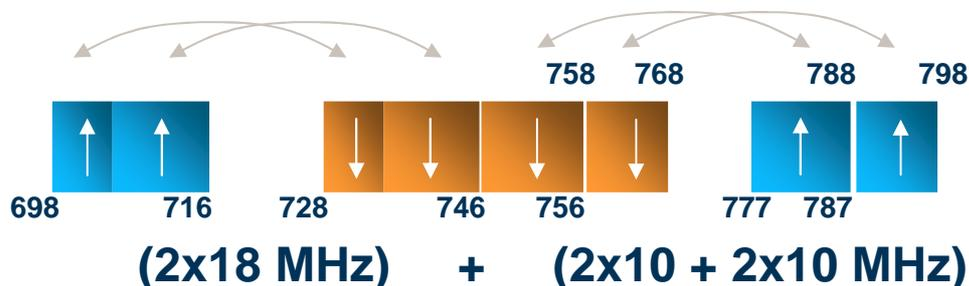
**Figure 2** The four frequency bands specified in 3GPP (Bands 12, 13, 14, and 17) identified as the US700 arrangement. The maximum use of this arrangement with specifications in 3GPP is this 2x18 MHz + 2x20 MHz. However, today the actual 3GPP implementation is limited to band 13 (primarily Verizon) and band 17 (primarily AT&T).
